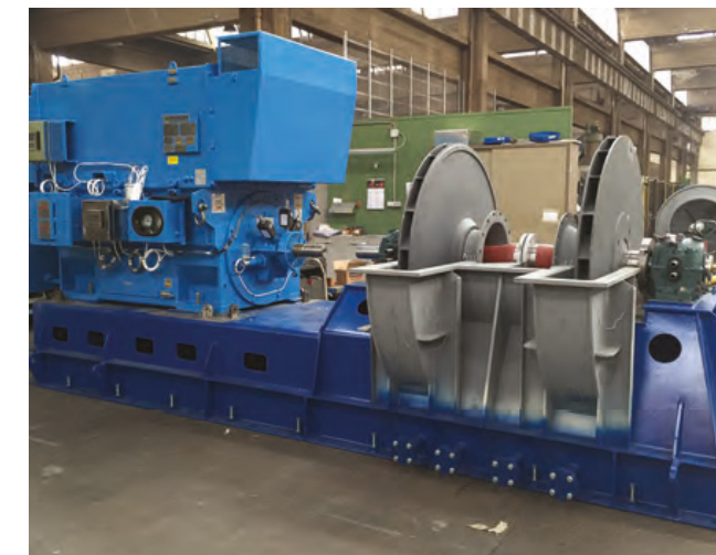
◆ FORMALDEYDE GAS BLOWER
