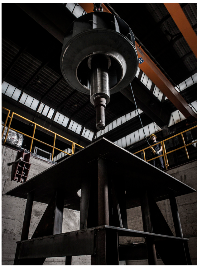
Figure 2. A fan's rotor being assembled at Boldrocchi's Italian workshop.
