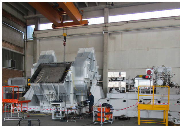
Figure 4. A fan undergoing a functional test at Boldrocchi's workshop near Milan, Italy.
