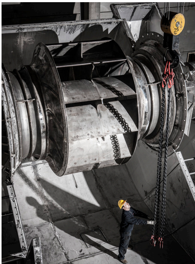
Figure 2. Granulator scrubber exhaust fan being mounted at Boldrocchi's in-house manufacturing facilities in Italy.
