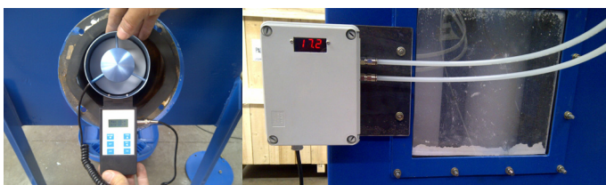
Figure 4. Flowrate setting and differential pressure measurement.
