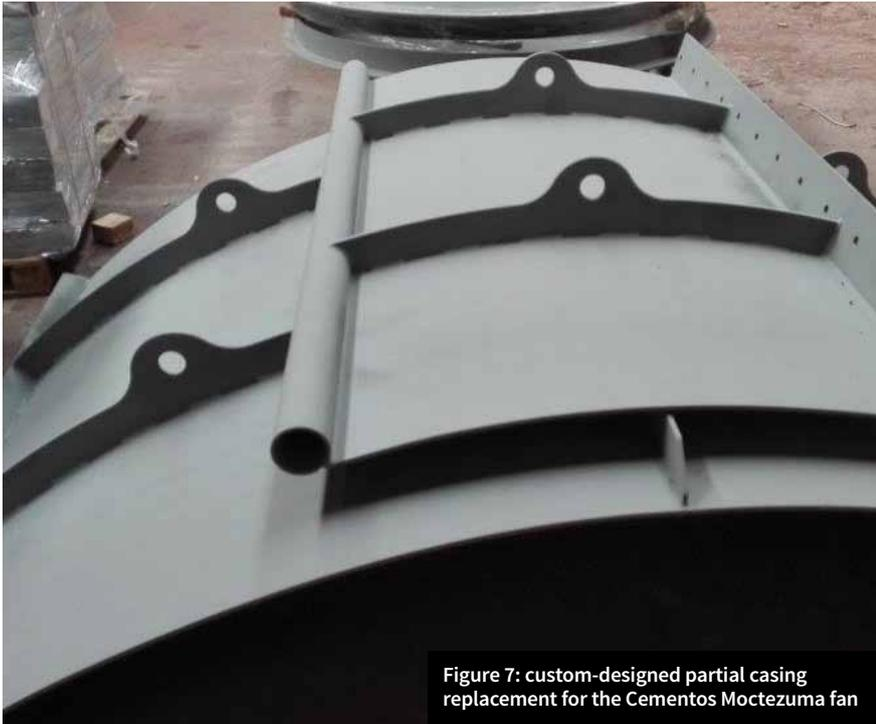
Figure 7: custom-designed partial casing replacement for the Cementos Moctezuma fan
